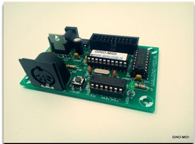
In order to minimize the wiring from the main PCB to the keyboards and the stops panel, the decoder circuits are accommodated at the keyboards and their matrix, and the main board and the decoder boards are connected to each other by the GINO-bus.
