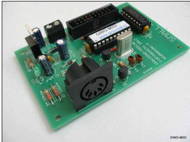
The MIDI-signal from the TXD-pin on the microprocessor is inverted by Q2 (BC547 or BC547B), and then transmitted through Q1 to the 5-PIN MIDI-connector. From decoder IC1A only the half is used. This is an address-decoder that decides which one of the 4 ports (manual, switches, and pedal) shall be read.
